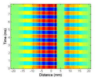
Figure 11. Intensity versus distance and time of chopped laser beam as imaged by LIDA.
