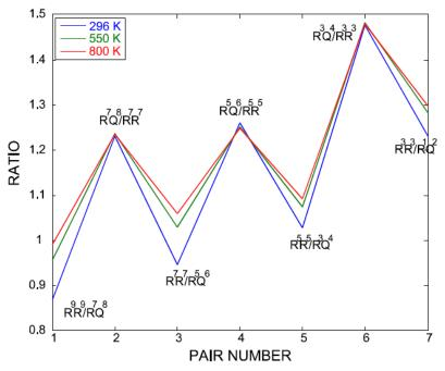
Figure 6. Temperature dependence of line pair ratios.
