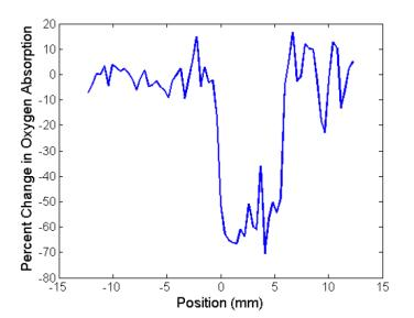
Figure 9. Depletion of oxygen as seen by the imaging array at the exit of the glass tube. Nitrogen gas is flown into the tube. Position between 0 and 6 mm is the glass tube.
