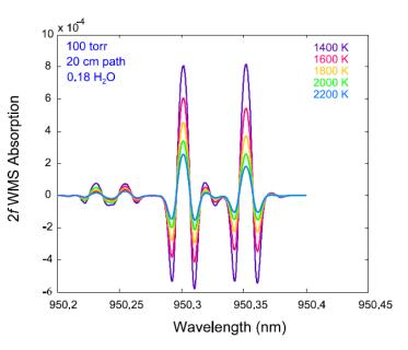
Figure 4. Potential line pair of water near 950 nm used for temperature and concentration measurements.
