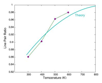
Figure 17. Temperature determined from line pair ratios using oxygen spectra. Solid curve is computed results. Symbols are experimental data.
