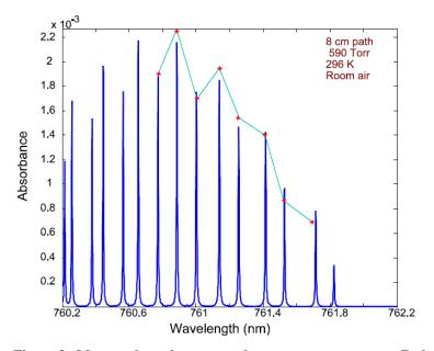
Figure 3. Measured and computed oxygen spectrum. Red markers denote measured positions and absorbances of sample.
