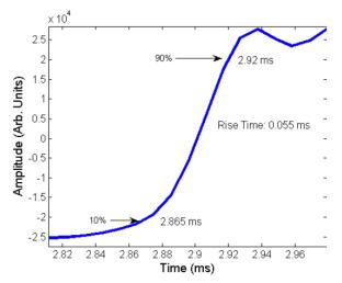
Figure 13. A section from the plot shown in Fig. 12 at 2.9 ms. The rise time is 0.055 ms.
