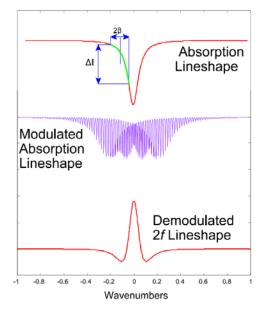
Figure 2. Generation of wavelength modulation spectroscopy (WMS) spectrum from transmission line shape.
