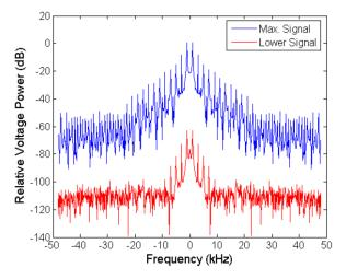
Figure 14. Plot showing the power spectrum of two pixels at about 2 mm (blue) and -21 mm (red) on the array detector.
