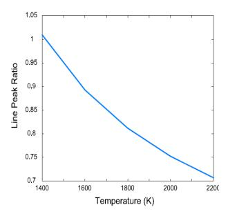
Figure 5. Line pair peak height dependence as a function of temperature.
