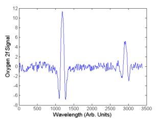
Figure 16. Sample oxygen 2*f* spectra collected by detector element No. 40.
