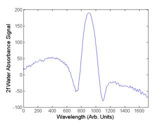
Figure 15. Sample water vapor 2*f* spectrum collected by detector element No. 40.
