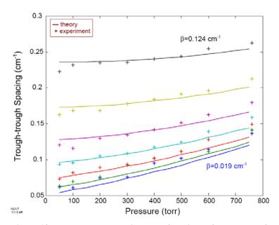
Figure 18. Trough separations as function of pressures for range of modulation depths.
