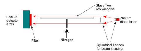
Figure 8. Schematic of the experimental apparatus used to test resolution and measurement of gas profiles. Nitrogen gas is continuously flown into the glass tee.
