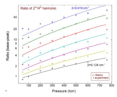
Figure 19. Peak height ratios for n=2 to n=4 WMS signals as a function of pressure for various modulation depths
