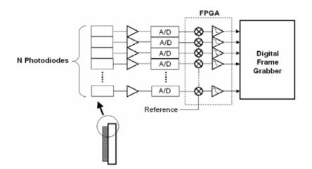
Figure 1. Schematic diagram of imaging sensor. Signal from each photodiode is sent to a transimpedance amplifier, programmable gain amplifier, 24-bit A/D converter, field programmable gate array (FPGA), and computer via a digital frame grabber.
