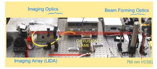
Figure 10. Test setup for testing the imaging sensor.
