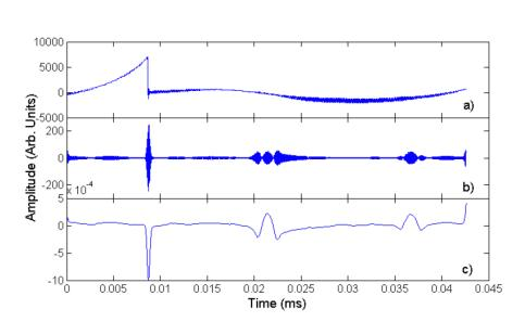
Figure 7. Steps required to process the data from LIDA for imaging wavelength modulation spectroscopy. (a) shows the raw data from LIDA; (b) shows the in-phase 2f component of the signal only; (c) is the demodulated 2f showing oxygen absorption features at 0.21 and 0.37 msec.
